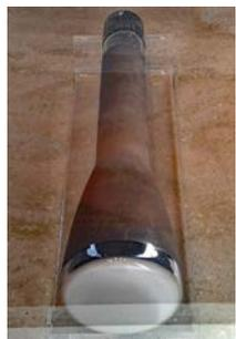
Freddie Williams applied for a patent on a Cathode-Ray Tube (CRT) storage device on Dec. 11, 1946. The CRT, used as computer memory to electronically store binary data, later became known as the [Williams tube](#) or Williams-Kilburn tube. The Williams tube stored only 128 40-bit words.
