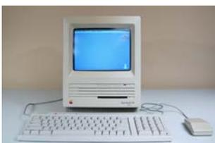
Launched in 1989, the Macintosh SE/30 was powered by a Motorola 60030 CPU, had 128Kb RAM, a built-in hard drive and a 1.4Mb floppy that could read PC disks. The Macintosh SE/30 sold for 2 years (1989-1991). It was the fastest and most expandable of Apple's black and white compact computers.
