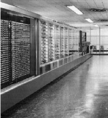
C.D Lake, H.H. Aiken, F.E. Hamilton, and B.M. Durfee filed a calculator patent for the Automatic Sequence Control Calculator, commonly known as the Harvard Mark I on February 8, 1945. The Mark I was a large automatic digital computer that could perform the four basic arithmetic functions and handle 23 decimal places. A multiplication took about five seconds.
