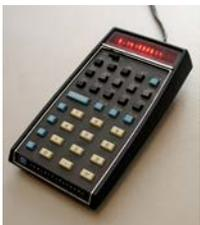
Perhaps marking the end of the slide rule, the 1st scientific hand-held calculator (HP-35) was introduced for \$395 (1972).
