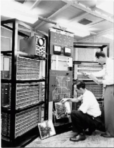
AT&T Bell Laboratories announced the completion of the first fully transistorized computer, TRADIC (1955). TRADIC, which stood for **TR**Ansistor **D**igital **C**omputer, contained nearly 800 transistors, which replaced the standard vacuum tube and allowed the machine to operate using less than 100 watts; one-twentieth the power of a comparable vacuum tube computer.
